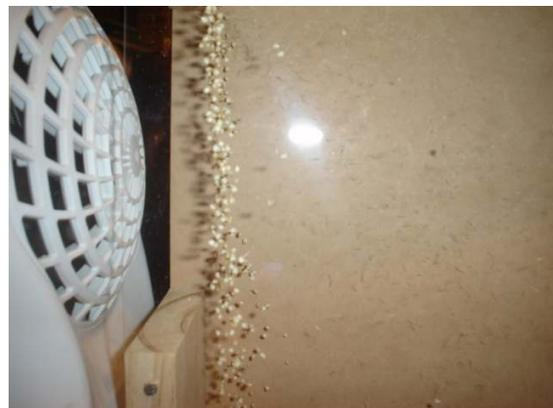
The close up photo shows the roots and shoots being blow further than the grain.
