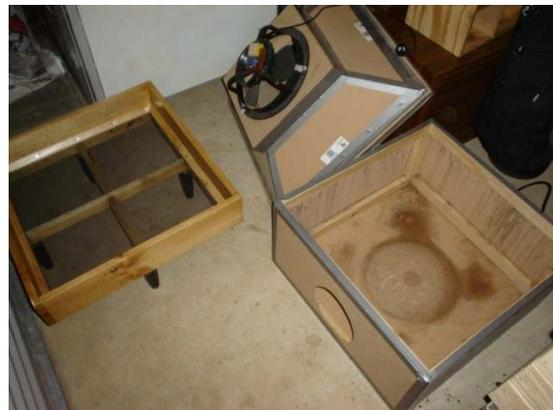
For germination I have constructed a dual purpose unit that also acts as the kiln. It is constructed out of pine, MDF and flywire screen and has three components; the base, the tray, and the fan.
